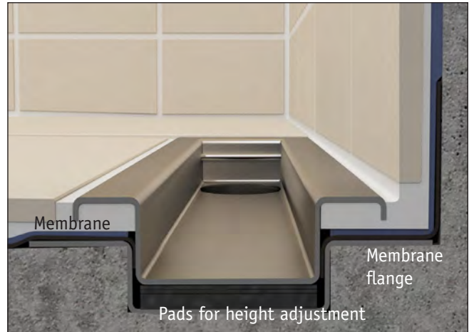
Tiles and liquid membrane
