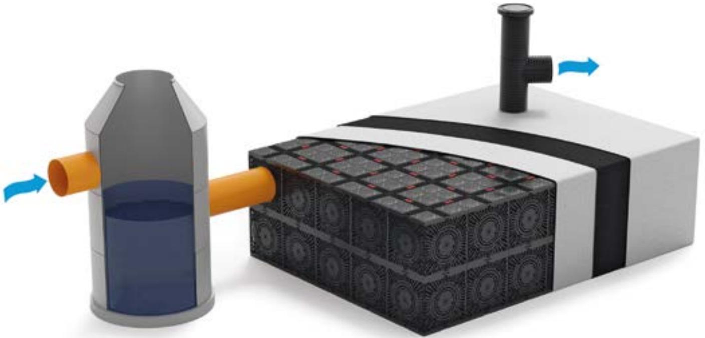
The rainwater running off from roofs or other surfaces and harvested for reuse is always channeled through a suitable pre-treatment stage before it can enter the storage tank. The water is conveyed into the Aquabox basin through one or more inlet pipes and is extracted when necessary with a pump housed in a suitably placed Aquabox Cube shaft.
