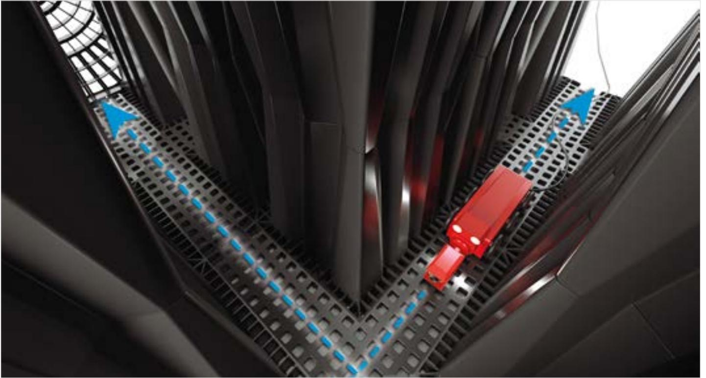
Each Aquabox module is formed by coupling two semi-modules. The system is composed of a series of modules joined by snap-lock clips and confined by lateral grids and upper closing covers: all these elements together create structural voids suitable for underground rainwater management.
