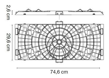
$<sup>^{\</sup>star}$  in consideration of the recycled material the measurements must be considered with a tolerance of  $\pm$  1.5%.
