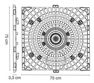
$<sup>^{\</sup>star}$  in consideration of the recycled material the measurements must be considered with a tolerance of  $\pm$  1.5%.
